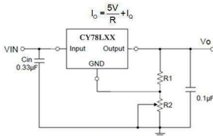
**Fig.3 Adjustable Output Regulator**
