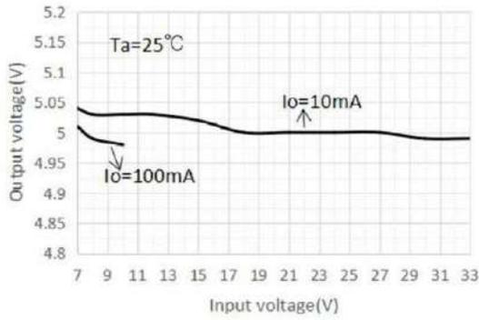
**Output Voltage vs. Load**
